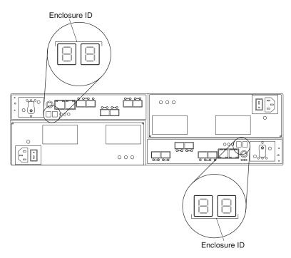
Figure 24. Storage subsystem seven-segment enclosure IDs
